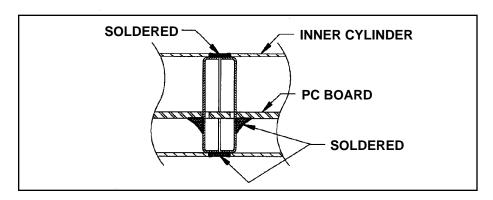
The soldered ground path technique provides much more stability to a trap notch over the life of the trap, than the separate cylinder design, held together through a mechanical fit.
